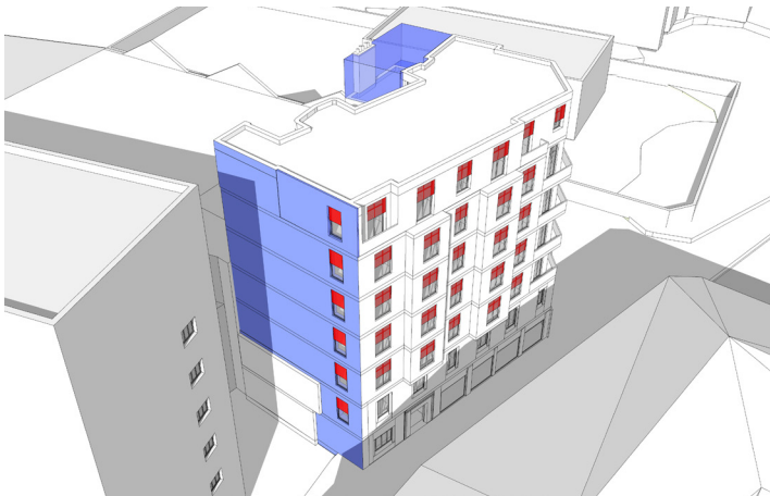
View from rue des Amandiers - Sun protection and over-elevation
